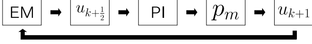
Fig. 5. The computational scheme for computing physiological parameters from the PET data. These parameters are computed via a two-step procedure containing the standard EM algorithm and a parameter identification (PI) process.
